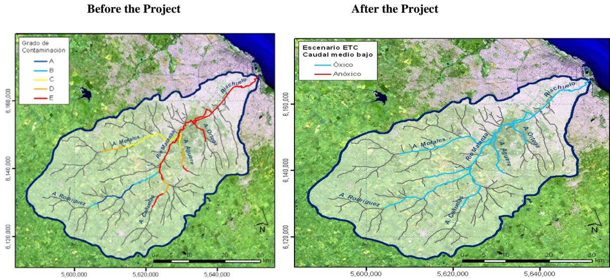
Note: The extent of contamination depending on current levels of dissolved oxygen (DO) along the extension of the river (from the lowest, A, to the highest, E). The river is currently in a persistent anoxic condition due to oxygen depletion especially in the proximity to the delta where MR flows into the de la Plata River. Stretches of the river with anoxic conditions are denoted in red.
